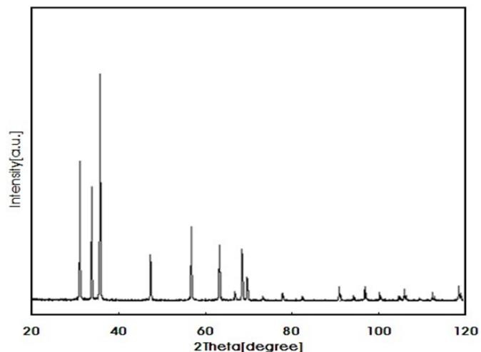
Figure 3. The X-ray powder diffraction (XRD) curves of Nano-crystalline ZnO (Adapted from Iranian Nano-materials Pioneers Company's catalog).
