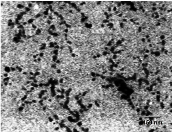
Figure 1. TEM image of ZnO NPs from stock suspension.
