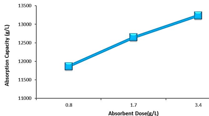
Figure 9. Adsorption capacity of Ag-rGO nanocomposite against coliform bacteria at concentrations of 0.8, 1.7 and 3.4 g/L of nanocomposite and  $96 \times 10^4$  CFU/mL of bacterial suspension. Minimum and maximum removals were observed at concentrations of 0.8 and 3.4 g/L, respectively.
