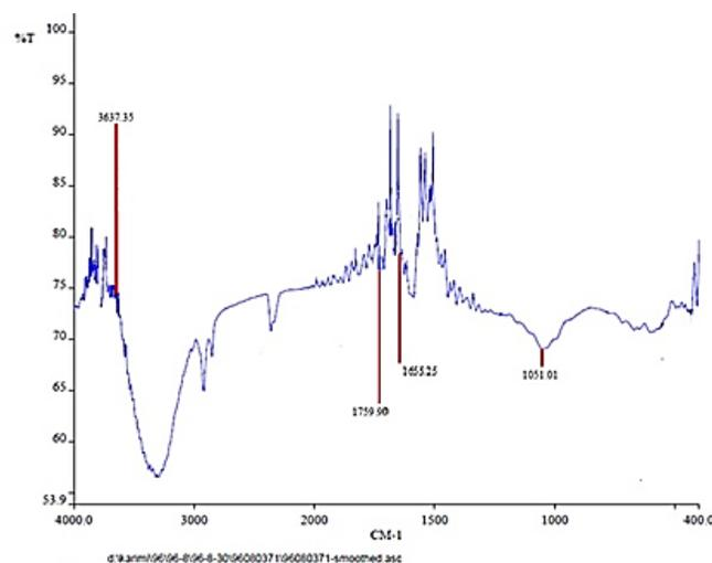
Figure 2. FT-IR spectrum of Ag-rGO nanocomposite: the peaks of OH, C=O, C-O-C and C=C bonds appeared at 3637, 1759, 1051, and 1655  $\text{cm}^{-1}$ , respectively.
