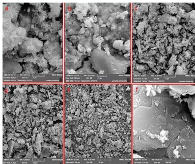
Figure 1. Different magnifications of SEM image of Ag-rGO nanocomposite.
