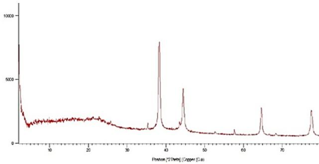
Figure 3. XRD pattern of Ag-rGO nanocomposite: the peaks shown in 400-800 nm confirm the proper formation of nanoparticles.
