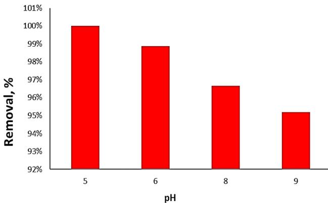
Figure 4. The effect of pH on the removal of coliform bacteria from aqueous solution by Ag-rGO nanocomposite at pH = 5, 6, 8, and 9. The minimum and maximum removals were observed at pH 5 and 9, respectively.
