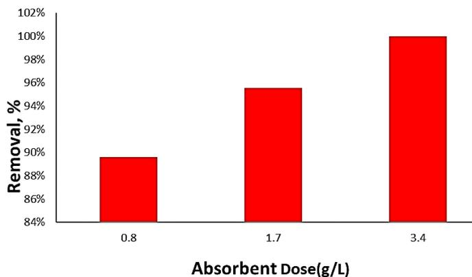
Figure 8. The effect of nanocomposite dose on the removal of coliform bacteria from aqueous solution by Ag-rGO nanocomposite at concentrations of 0.8, 1.7 and 3.4 g/L of nanocomposite and  $96 \times 10^4$  CFU/mL of bacterial suspension. Minimum and maximum removals were observed at concentrations of 0.8 and 3.4 g/L, respectively.
