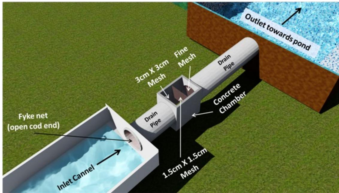
Figure 4. Photographic image of the suggested 'Modified Vertical Barrier (MVB).
