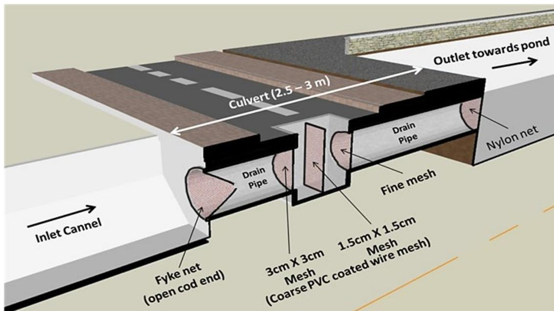
Figure 5. Cross section of the suggested 'Modified Vertical Barrier (MVB).
