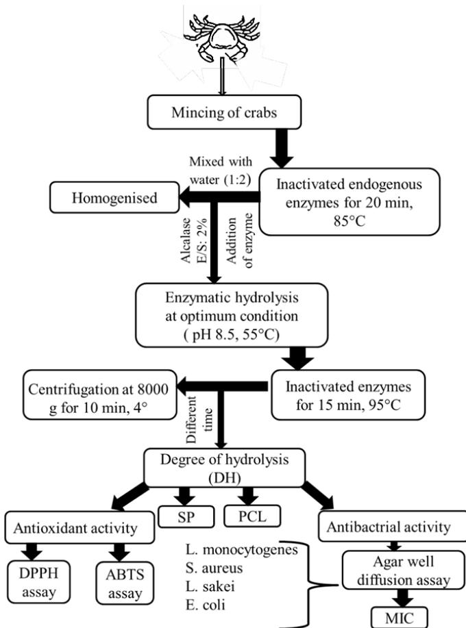
Figure 1. Flow diagram of the crab hydrolysis process and investigation of antioxidant and antibacterial activities.
