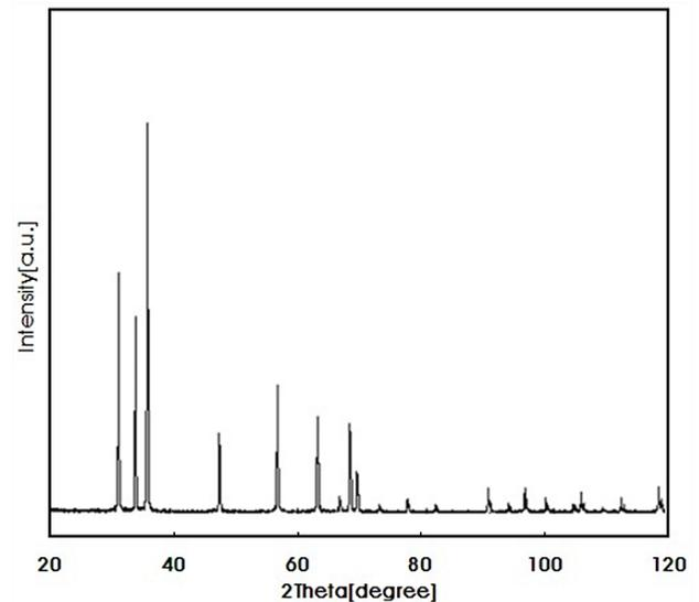
Figure 3. The X-ray powder diffraction (XRD) curves of Nano-crystalline ZnO (Adapted from Iranian Nano-materials Pioneers Company's catalog).
