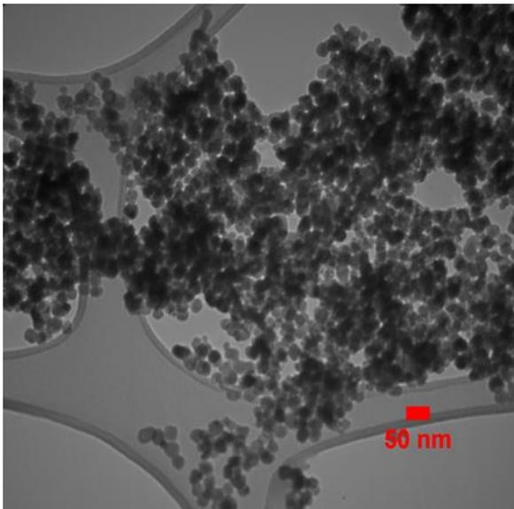
Figure 3. TEM micrographs of the Nano-ZnO powders (Adapted from Iranian Nano-materials Pioneers Company's catalog).
