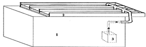
Figure 1. Schematic feature of the used recirculating aquaculture system: 1. the fish tank 2. The hydroponic troughs 3. The water pump (Rafiee and Saad, 2005).
