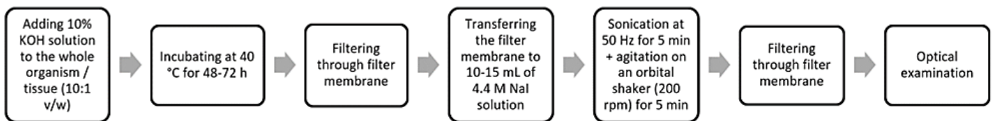
Figure 3. Flow diagram of microplastic extraction protocol (Karami et al., 2017)
