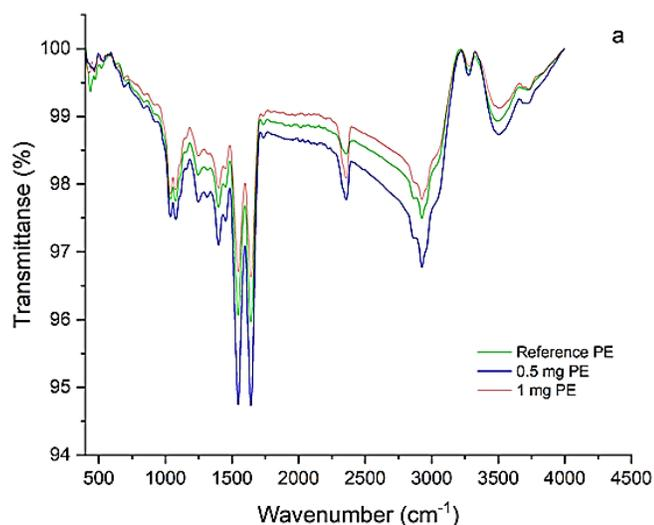
Figure 1. Fourier infrared spectroscopic spectrum related to hemolymph (a) samples to detect PE-MPs.
