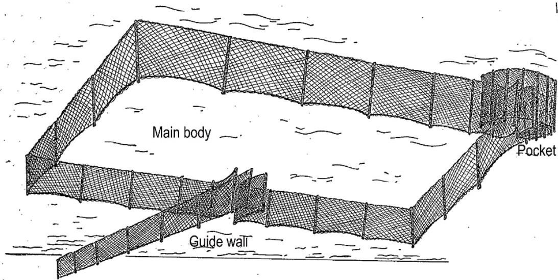
Figure 1. Schematic drawing of a Moshta showing its three main parts.
